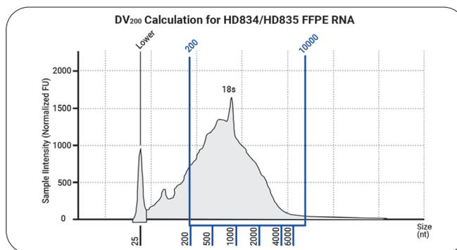
Figure 2: Typical TapeStation electropherogram trace for HD834/HD835 FFPE RNA, showing DV<sub>200</sub> region (200–10000 nt) in blue (measured DV<sub>200</sub>=83%), as measured with the High Sensitivity RNA ScreenTape® Assay (Agilent™).
